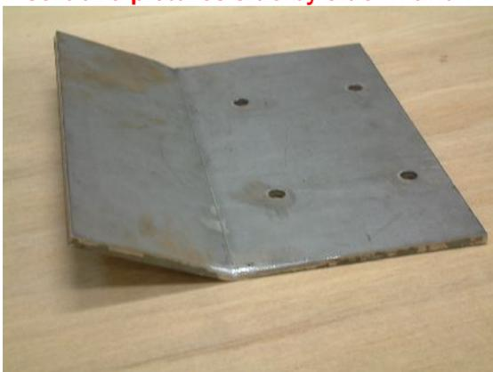
The Shoe, depending upon the profile chosen, produces either a tapered safety edge along the side of the road or a longitudinal center lane joint. The Shoe is attached to the bottom of the Wedge with screws and lock washers.
