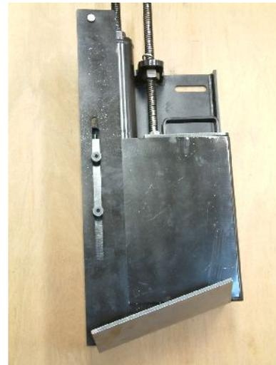
**Creating Safety Edge Slopes less than 30°.** In some cases, say for example because of rolling patterns that tend to push out the asphalt thereby increasing the slope angle that was initially created by the shoe, the operator may wish to create a slightly flatter angle so that the final result will tie in with a 30° slope.
