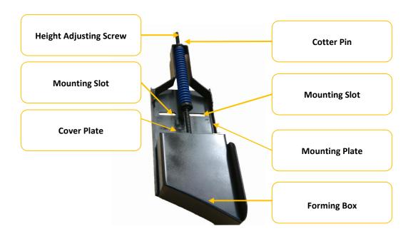
Mounting Slots are used for attaching the Mounting Plate to the screed extension of the paver.  $\frac{1}{2}$ " bolts, washers, lock washers and nuts are provided to mount the unit.
