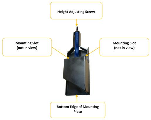
There are two Mounting Slots on the Advant-Edger Mounting Plate. They are symmetrical in size and location. The unit pictured above is in the Mounting Position. Note that the Forming Box has been raised to its highest level and it is flush with or slightly above the bottom edge of the Mounting Plate.
